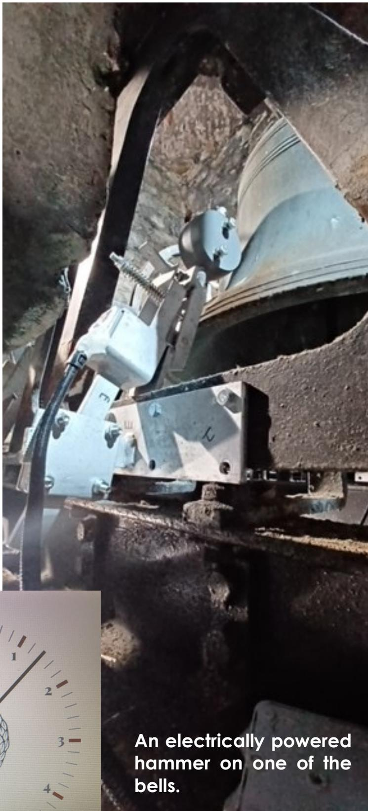
**An electrically powered hammer on one of the bells.**
